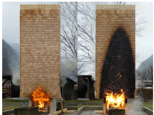
A fire test of the shingle facade
